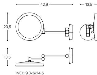
**LED lighting**, touch switch, 5 x magnification, hanging design, 100 - 250 V external power supply / built-in power supply. Wall-mounted model that can be adjusted to different angles.
